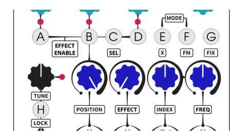
**A, B, D: EFFECT ENABLE** Enables the effect for the associated wave slot, **A, B** or **C**.
