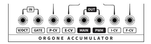
**V/OCT:** Standard 1 volt per octave input for pitch. Over 4-octave resolution. Typical inputs: CV keyboard, LFO, sequencer CV output.
