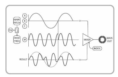
Three oscillators are mixed in a ratio controlled with **POSITION**. The output amplitude-modulates the **MODULATION** oscillator, which is also synced to the main pitch.
